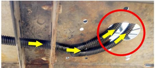
6. Route the taillight leads to the holes that were cut out for the taillights. The shorter lead will go over the driver side inner fender. The longer lead will go behind the bat-
