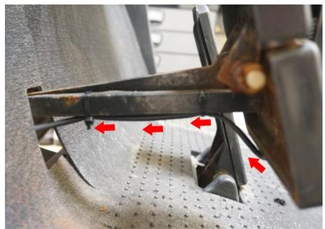
4. Connect the brake pad to the deluxe wire harness. Use a cable tie to secure the wires to the existing wire harness in the channel. Make sure the wires are clear of any moving parts.
