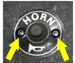
9. Install the horn button and decal using the Included Nut and Rubber Bumper Cover. Align the decal. Secure the decal with the (2) Rivets.
