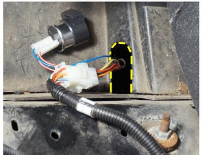
4. Run the turn signal wires down the steering column, through the access hole and into the dash area.
