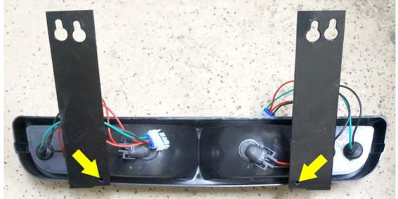
3. Install the light bar to the splash guard by sliding the slots at the top of the brackets over the bolts loosened in Step 1. There are two different slots. Select the one that aligns best.
