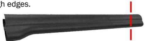
11. Snap the cover around the wires of the turn signal switch and the steering column.
