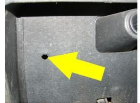
6. Locate the (2) pre-drilled holes for the rivets. If your cart has the mounting holes, they will be next to the horn button hole. Remove the floor mat over the holes with a 7/32" drill bit. If your cart does not have pre-drilled holes, follow Steps 7-8 below.
