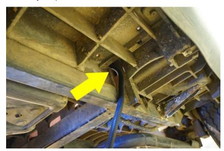
5. Make sure the battery connection leads are able to reach the battery pack. Set the leads to the side. They will be connected after completing the installation of the harness, lights and/or accessories.
